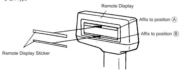
Affix the remote display stickers to the inner edge of the remote display sheet. (The sticker should be affixed on both the operator side and customer side)
